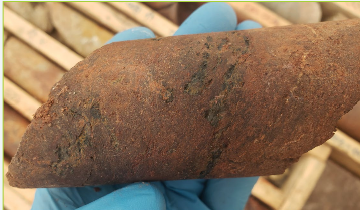
High-grade uranium (>1% U 3 O 8 ), drill hole AK21-001
